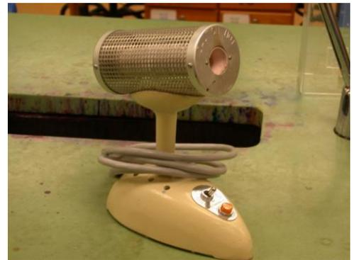
Figure 4: Incinerator
